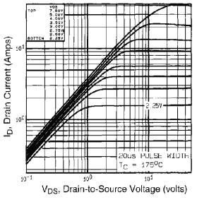
Fig. 2 - Typical Output Characteristics, T<sub>C</sub> = 175 °C
