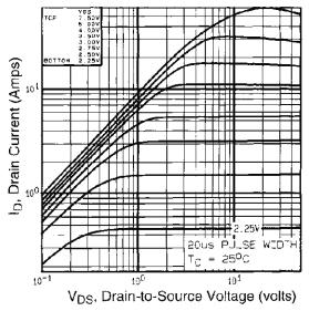
Fig. 1 - Typical Output Characteristics, T<sub>C</sub> = 25 °C
