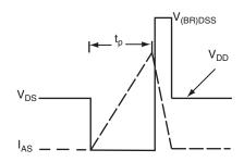
Fig. 12b - Unclamped Inductive Waveforms
