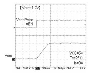
Fig.14 Soft start waveform
