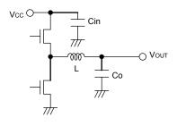
Fig.30 Input capacitor
