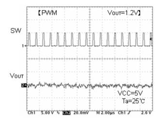
Fig.16 SW waveform Io=10mA
