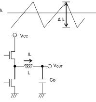
Fig.28 Output ripple current
