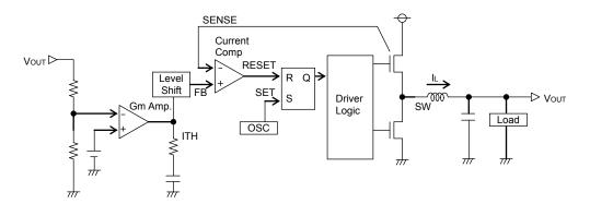
Fig.19 Diagram of current mode PWM control
