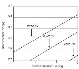
Fig.35 minimum input voltage in each output voltage
