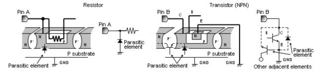
Fig.38 Simplified structure of monorisic IC
