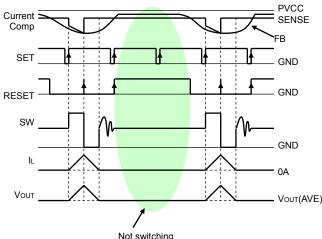
Fig.21 SLLM<sup>TM</sup> switching timing chart
