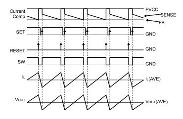
Fig.20 PWM switching timing chart
