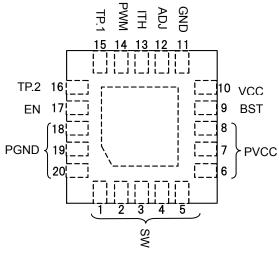
Fig.2 Pin configuration
