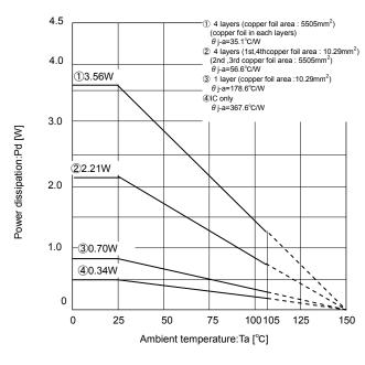
Fig.27 Thermal derating curve (VQFN020V4040)
