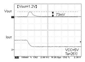
Fig.18 Transient Response Io=3→1A(10µs)
