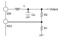
Fig.34 Determination of output voltage
