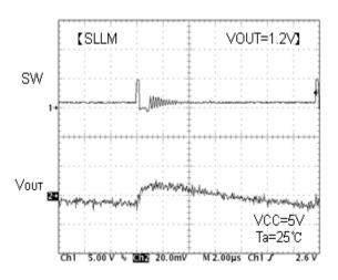
Fig.15 SW waveform Io=10mA
