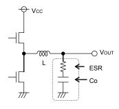
Fig.29 Output capacitor
