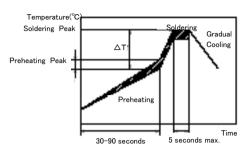
[Allowable Soldering Temperature and Time]
