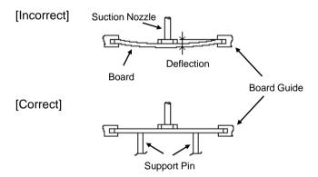
2.Dirt particles and dust accumulated between the suction nozzle and the cylinder inner wall prevent the nozzle from moving smoothly. This imposes greater force upon the chip during mounting, causing cracked chips. Also the locating claw, when worn out, imposes uneven forces on the chip when positioning, causing cracked chips. The suction nozzle and the locating claw must be maintained, checked and replaced periodically.
