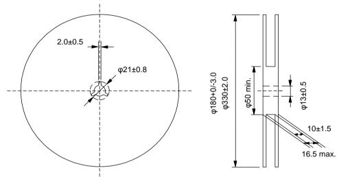
Fig.3 Taping Diagram
