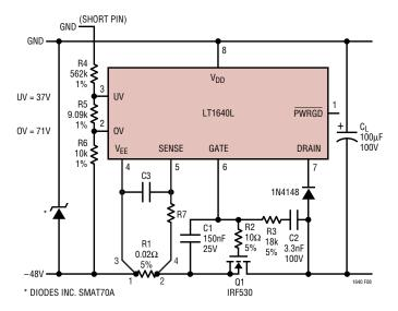
Figure 8. Extending the Short-Circuit Protection Delay
