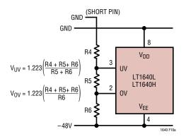
Figure 10a. Undervoltage and Overvoltage Sensing
