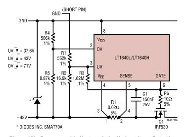
Figure 10b. Programmable Hysteresis for Undervoltage Detection
