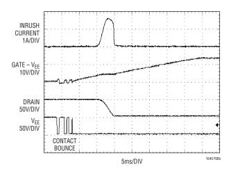
Figure 6b. Inrush Control Waveforms
