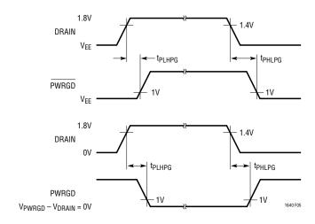
Figure 5. DRAIN to PWRGD/PWRGD Timing
