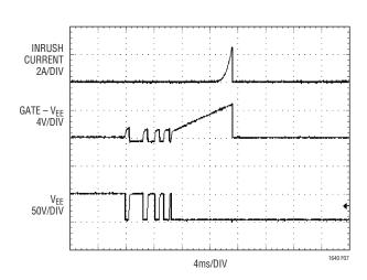
Figure 7. Start-Up Into a Short Circuit
