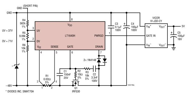
Figure 6a. Inrush Control Circuitry
