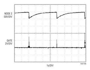
Figure 9. Automatic Restart After Current Fault
