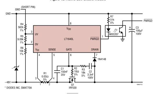
Figure 13. Using PWRGD to Drive an Optoisolator
