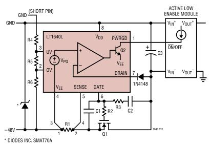
Figure 12. Active Low Enable Module
