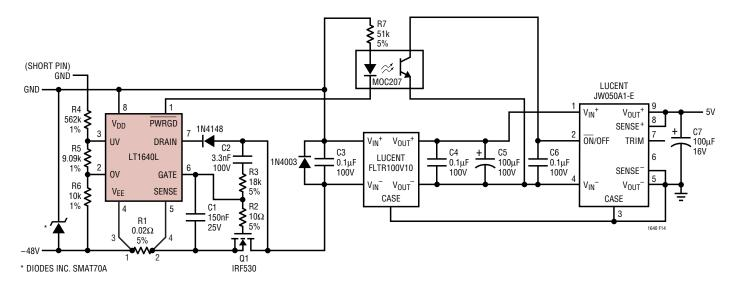
Figure 14. Typical Application Using a Filter Module
