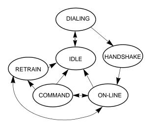
Figure 4. Modem State Diagram
