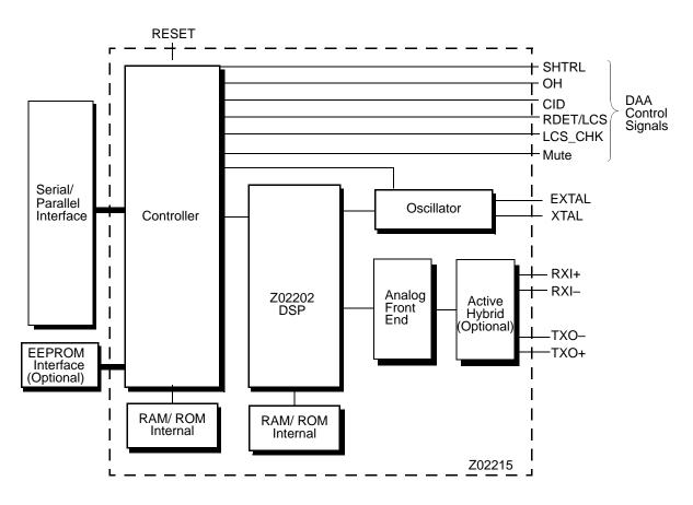
Figure 1. Z02215 Block Diagram
