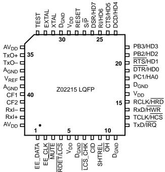
Figure 3. Z02215 44-Lead LQFP Pin Identification
