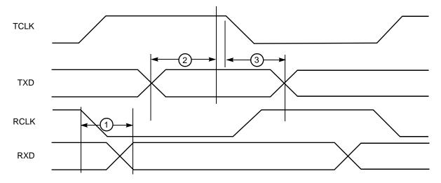
Figure 11. Serial Port Timing Diagram
