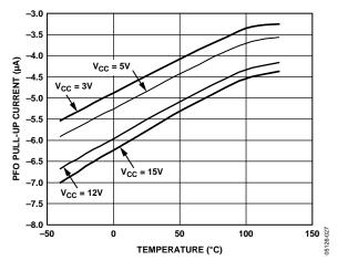
Figure 33. PFO Pull-Up Current vs. Temperature
