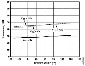
Figure 25. toff(ONLOW) vs. Temperature
