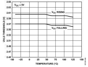
Figure 7. UVLO Threshold vs. Temperature
