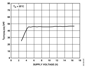
Figure 24. toff(ONLOW) vs. Supply Voltage
