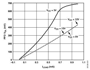
Figure 37. PFO Output Low Voltage vs. Load Current
