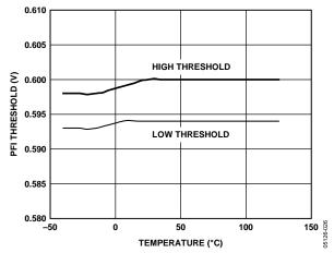
Figure 32. PFI Threshold vs. Temperature
