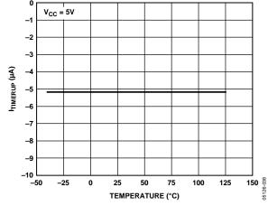
Figure 13. Itimerup (In Initial Cycle) vs. Temperature
