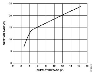
Figure 8. GATE Voltage vs. Supply Voltage
