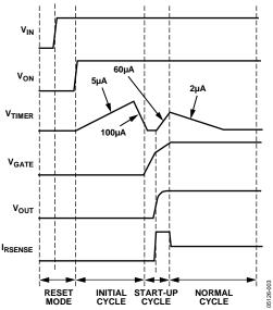
Figure 39. Power-Up into Capacitor
