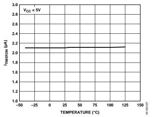
Figure 17. I<sub>TIMERDN</sub> (In Cool-Off Cycle) vs. Temperature
