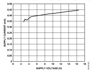
Figure 4. Supply Current vs. Supply Voltage (GATE Off)
