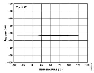
Figure 15. I<sub>TIMERUP</sub> (During Cct Breaker Delay) vs. Temperature
