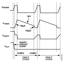
Figure 40. ADM1172-1Automatic Retry During Overcurrent Fault
