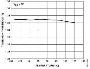
Figure 19. TIMER High Threshold vs. Temperature
