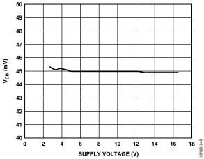
Figure 26. Cct Breaker Voltage vs. Supply Voltage
