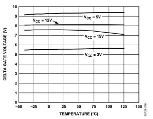
Figure 11. Delta GATE Voltage vs. Temperature
