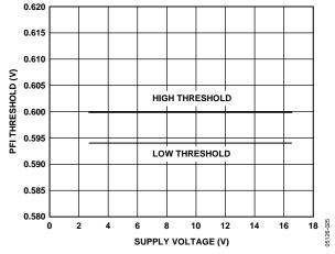
Figure 31. PFI Threshold vs. Supply Voltage
