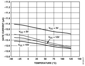
Figure 30. GATE Current (up) vs. Temperature
