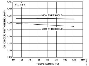
Figure 23. ON (ON-CLR) Pin Threshold vs. Temperature
