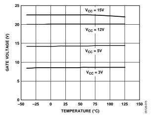
Figure 9. GATE Voltage vs. Temperature
