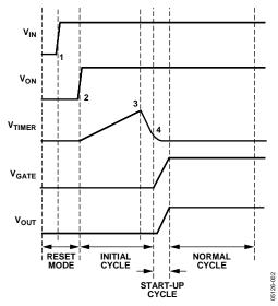
Figure 38. Power-Up Timing
