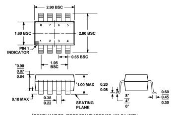
\*COMPLIANT TO JEDEC STANDARDS MO-193-BA WITH THE EXCEPTION OF PACKAGE HEIGHT AND THICKNESS. Figure 42. 8-Lead Thin Small Outline Transistor Package [TSOT] (UJ-8) Dimensions shown in millimeters
