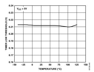
Figure 21. TIMER Low Threshold vs. Temperature
