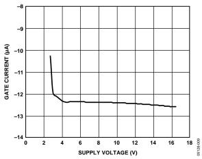
Figure 29. GATE Current (Up) vs. Supply Voltage
