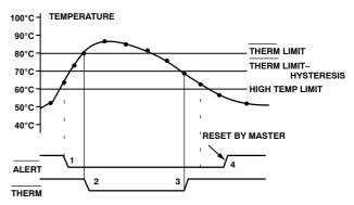
Figure 14. Operation of the ALERT and THERM Interrupts
