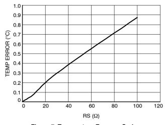
Figure 7. Temperature Error vs. Series
