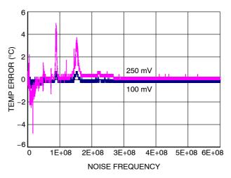
Figure 8. External Temp Error vs. Power Supply Noise
