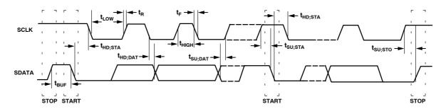
Figure 2. Serial Bus Timing
