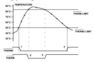
Figure 15. Operation of the THERM and THERM2
