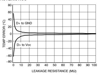
Figure 4. Temperature Error vs. PCB Leakage Resistance
