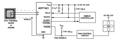
Figure 17. Typical Application Circuit
