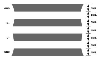
Figure 16. Typical Arrangement of Signal Tracks
