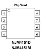
$\begin{array}{l} \mbox{PIN FUNCTION} \\ 1.I_{o} \ (Current Source) \\ 2.R_{s} \ (Scale Factor) \\ 3.V_{Lo} \ (Logic Output) \\ 4.GND \\ 5.R_{o} \ (One-Shot R,C) \\ 6.T_{h} \ (Threshold) \\ 7.V_{l} \ (Input Voltage) \\ 8.V+ \end{array}$
