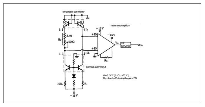
Figure 14. Temperature to Frequency converter
