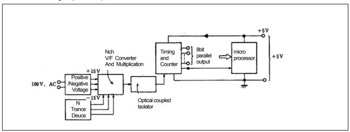
Figure 10. Connect to Micro Processor
