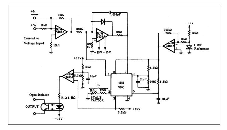
Figure 7. Opto-Isolated VFC
