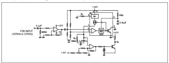
Figure 8. FSK demodulator
