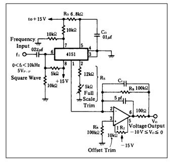
Figure 5. Single Supply Frequency-to-Voltage Converter
