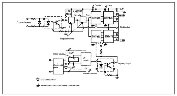
Figure 12. 8-bit ADC system (for 1-channel)
