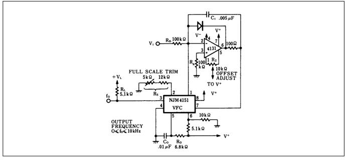
Figure 4. Precision Voltage-to-Frequency Converter
