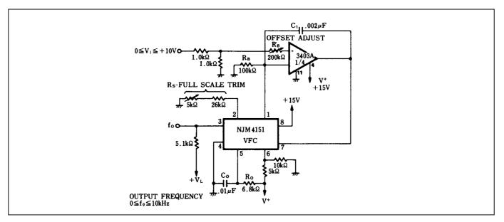
Figure 3. Precision Voltage-to-Frequency Converter Single Supply
