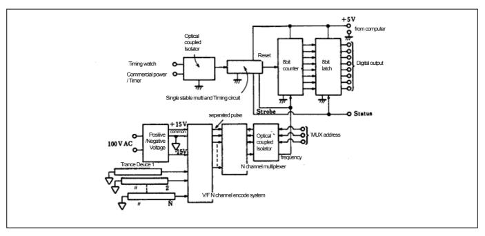
Figure 11. Multi channel ADC system
