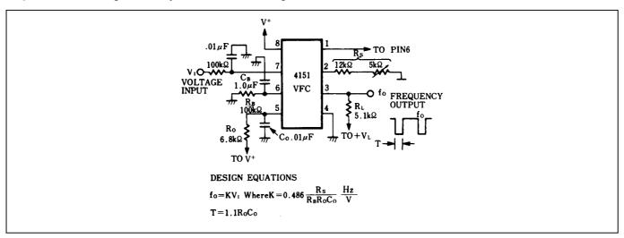
Figure 2. Single Supply Voltage-to-Frequency Converter
