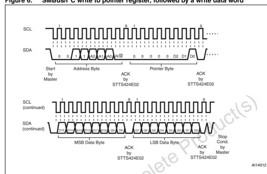
Figure 6. SMBus/I<sup>2</sup>C write to pointer register, followed by a write data word
