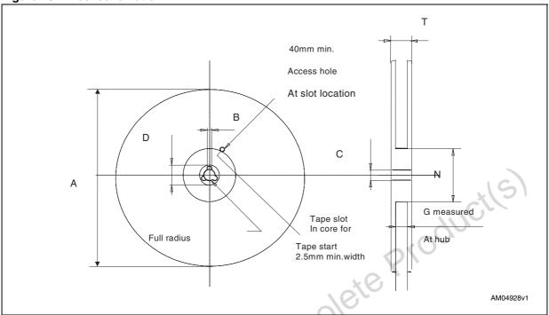
Table 31. Reel dimensions for 8 mm carrier tape - TDFN8 and DFN8 packages
