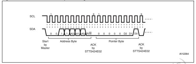
Figure 5. SMBus/I<sup>2</sup>C write to pointer register, followed by a read data word
