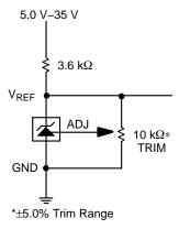
If the external trim resistor is not used, the "ADJ. PIN" should be left floating. The 10k trim potentiometer does not effect the temperature coefficient of the device.
