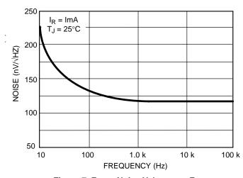
Figure 7. Zener Noise Voltage vs. Frequency
