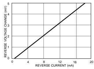
Figure 4. Change in Reverse Voltage vs. Reverse Current
