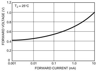
Figure 5. Forward Voltage vs. Forward Current
